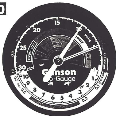
LATE VALVE TIMING: this is indicated by needle fluctuating between 5in and 10in at idle.
