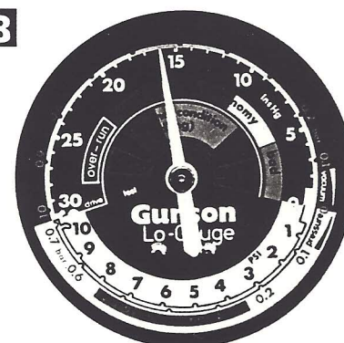
LATE IGNITION: a steady needle 2-3in below normal at tickover indicates retarded ignition.
