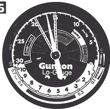
LOW VACUUM: if needle floats between 15-18in mixture is rich. Check air cleaner and float level.
