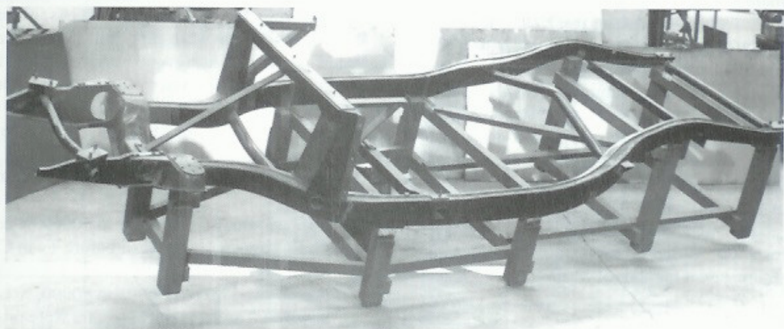
Chassis Jig for CKD frame construction Photo: Courtesy Piers Hubbard
