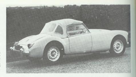
The hood and side curtains are a snug fit and follow closely the contours of the body. no exterior door handle. Three large windows at the back of the hood are made of flexible Vybak. Bumper over-riders are standard
